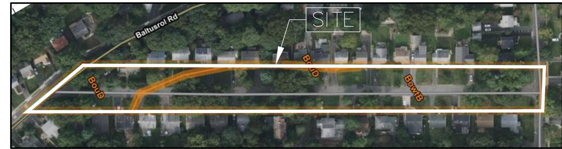
SOILS MAP SCALE: 1"=150' MAP SOURCED FROM USDA WEB SOIL SURVEY THE SITE IS MADE UP OF: BouD (BOONTON-URBAN LAND COMPLEX, 15 TO 25 PERCENT SLOPES) BowB (BOONTON-URBAN LAND COMPLEX, TERMINAL MORAINES, 0 TO 8 PERCENT SLOPES)
