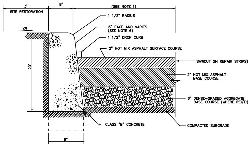
NOTE: 1) IN AREAS WHERE EXISTING PAVEMENT IS TO REMAIN, A 2" WIDE PAVEMENT REPAIR STRIP SHALL BE CONSTRUCTED ALONG PROPOSED CURB. THE FOLLOWING ITEMS OF WORK WITHIN THE REPAIR STRIP ARE INCLUDED UNDER 9" x 20" CONCRETE VERTICAL CURB:
