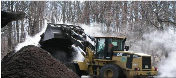
*A front end loader is used to turn the windrows and to move the finished composted material.*
