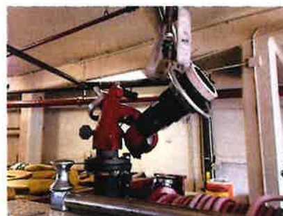
Image 23: Apparatus Bay Clearance Problems
