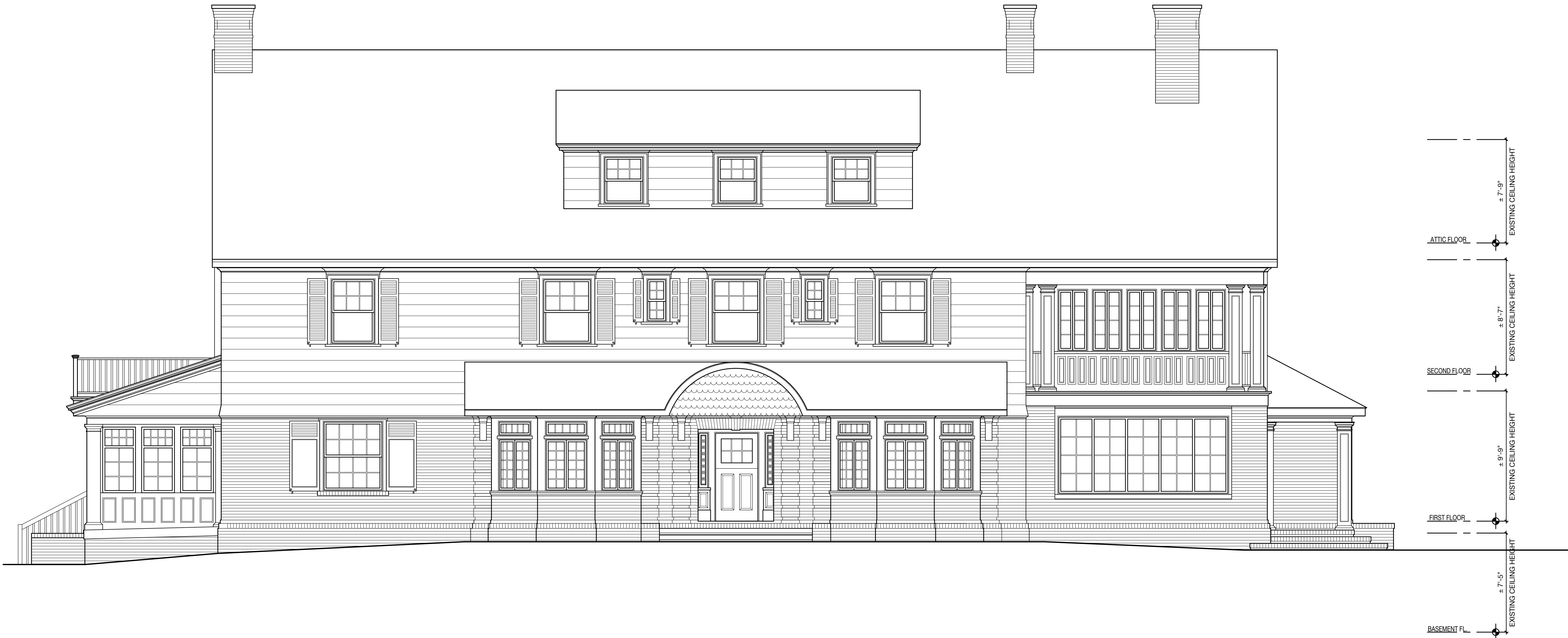
1 EXISTING FRONT ELEVATION SCALE: 1/4" = 1'-0"
