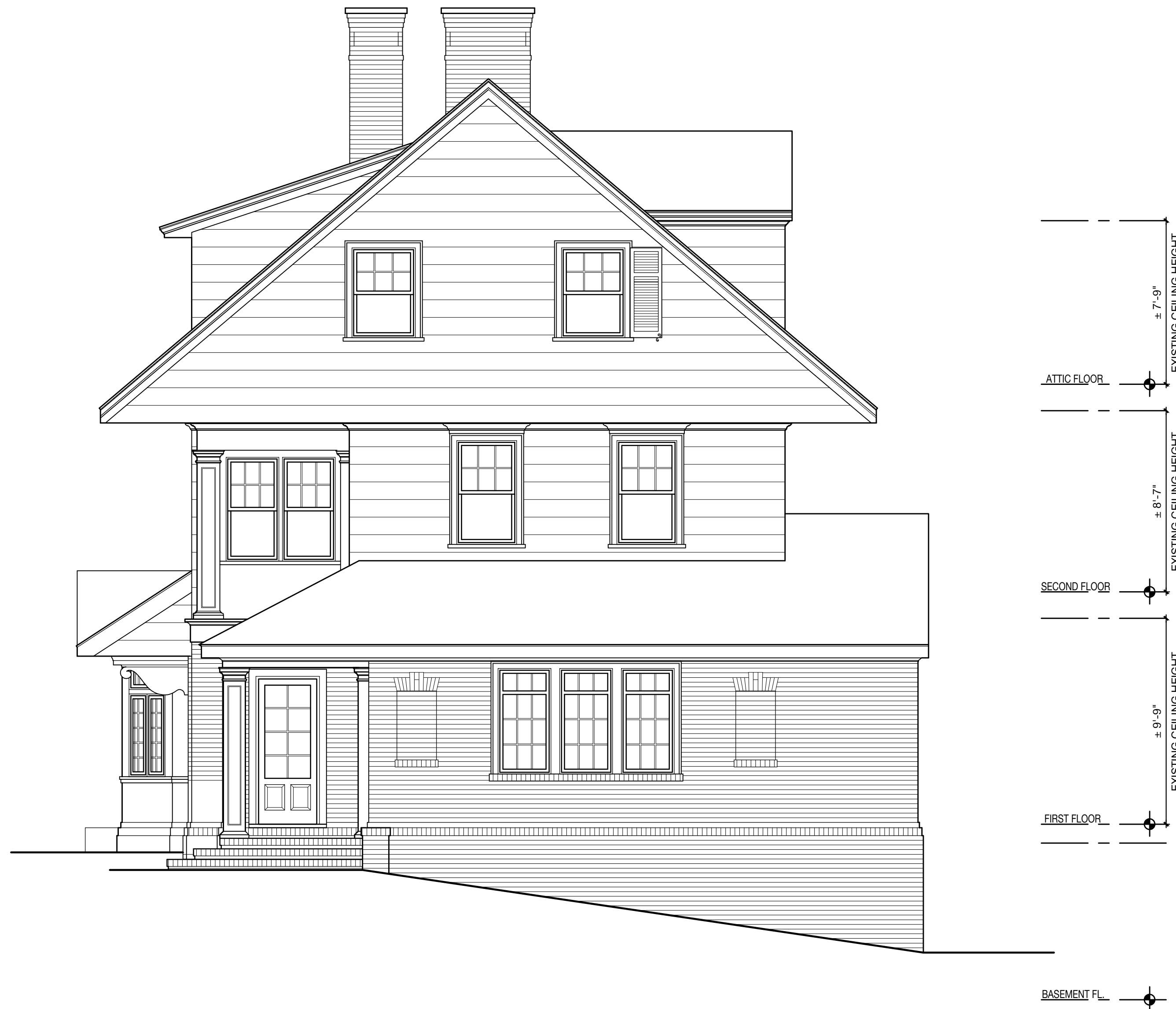
1 V-13 EXISTING RIGHT SIDE ELEVATION SCALE: 1/4" = 1'-0"
