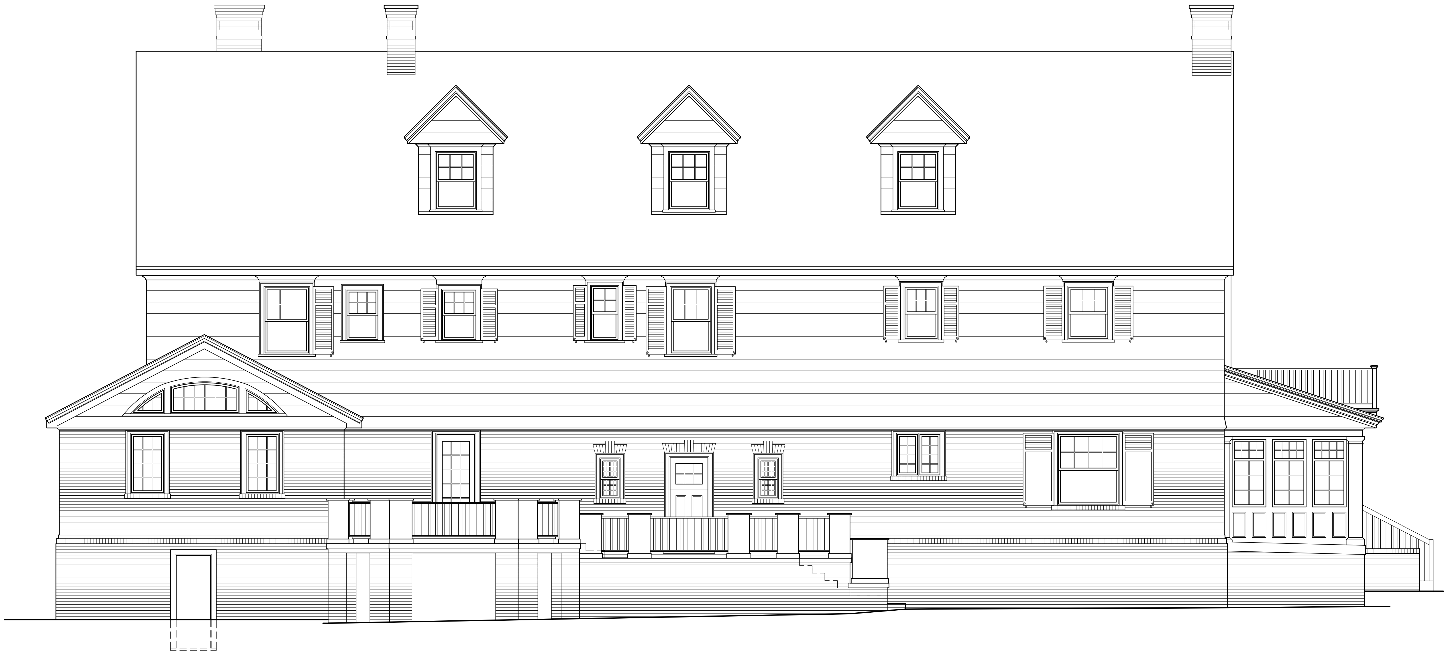
1 V-12 EXISTING REAR ELEVATION SCALE: 1/4" = 1'-0"
