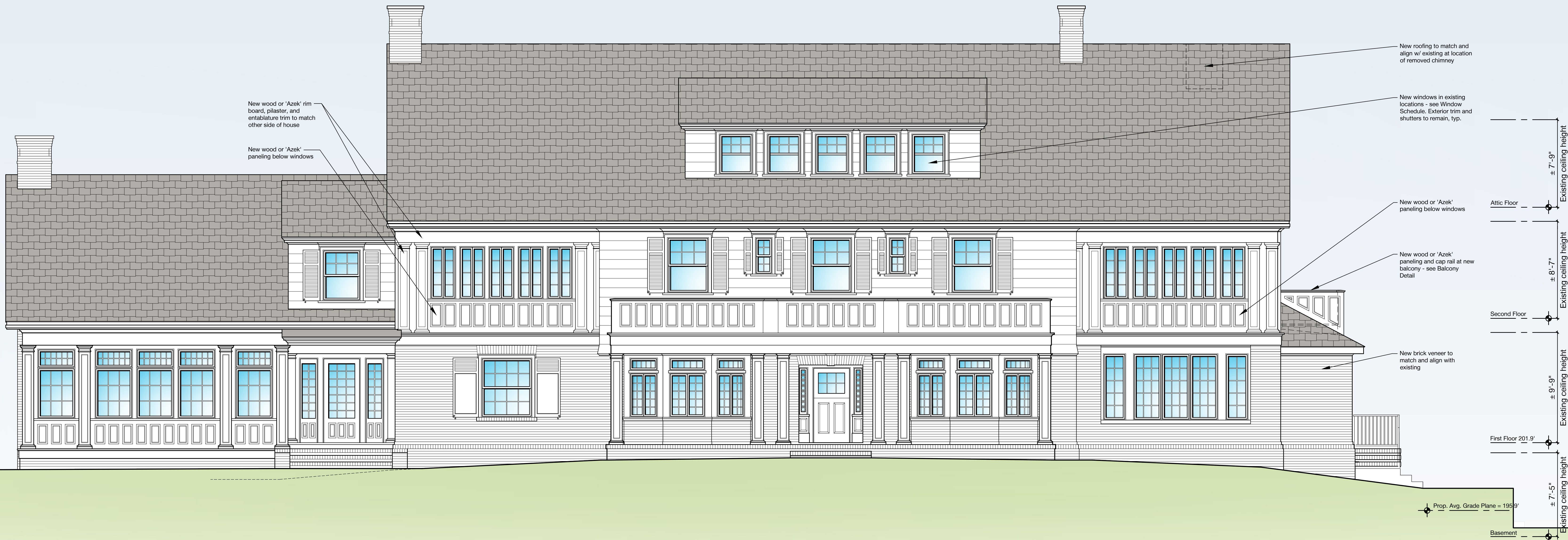
2 PROPOSED FRONT ELEVATION SCALE: 1/4" = 1'-0"
